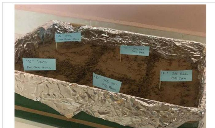
Figure 4: Samples were buried into wet soil boxes, and flags with their names were used to sign them and to know each sample.
